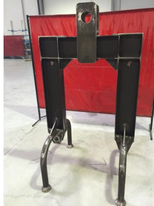
Spreader – AREVA SWL 10 tons
