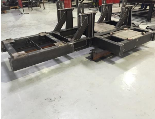
Frame for an inspection machine – AREVA Dimensions 3000x1500x700mm, Weight 680 kg
